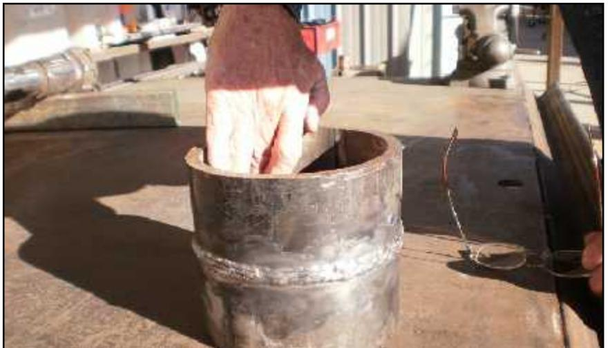
*SMOOTH JOINT: The two pieces of pipe are now one, and ready to be cleaned, polished, and cut into strips called 'coupons'.*
