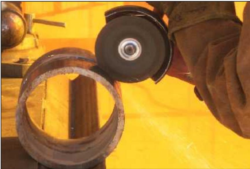
*The two pieces of pipe that are now one are cleaned and polished. Then they will be cut into multiple pieces—strips across the weld joint to be used for the final step of the 6G test.*
