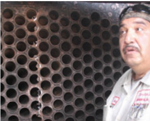
Standing in the smokebox next to the front tube sheet, a Chardans Mechanical boiler specialist begins tube removal instruction. The tubes are swaged or crimped at this end. Each tube must be collapsed at this end, cut free at the rear tube sheet, and pulled out through the smokebox.
