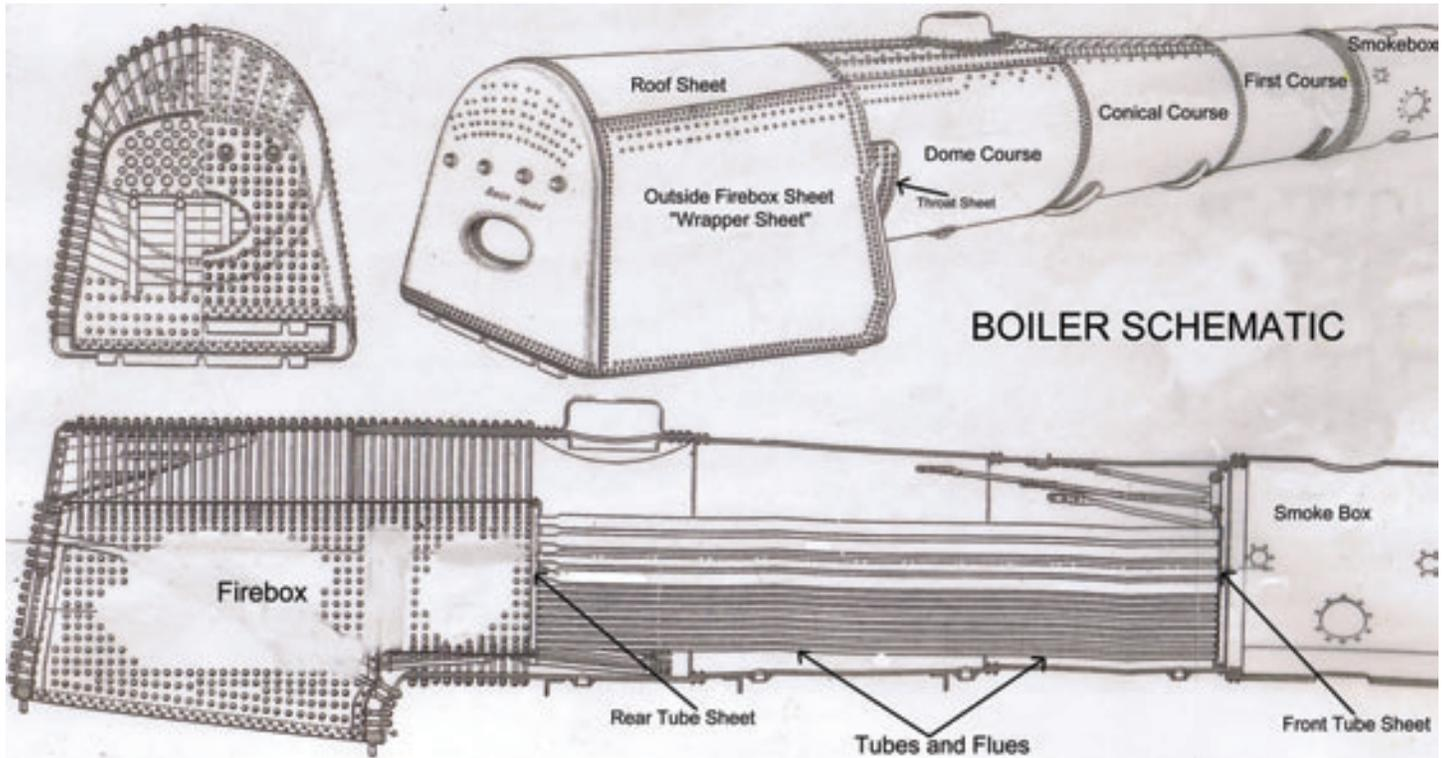
*This schematic is similar, but not an exact representation of the 2926 boiler. However, it is close enough to be used here to depict the challenging job of pulling the flue tubes. The pictures below show the removal process.*
