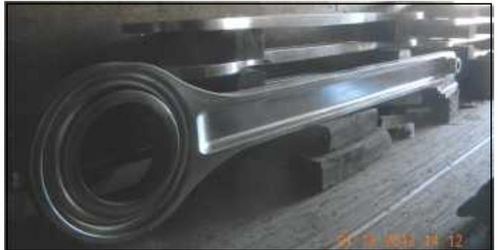
*The highly polished side rods are stored inside one of our storage containers. Once their large roller bearings are returned for the Timken plant in South Carolina, they will be taken out of storage and reinstalled.*
