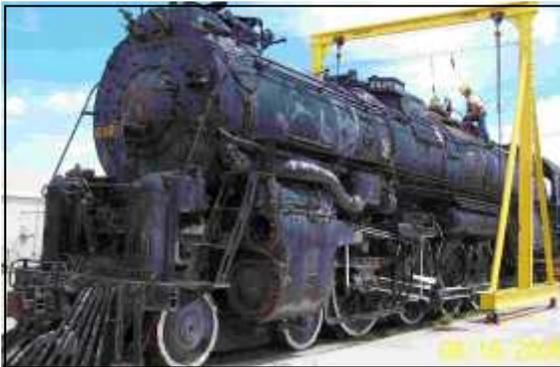
*Before removal of outer skin, asbestos, appliances, piping etc., 2926 reveals rust and other results of years of abuse, exposure, and neglect.*
