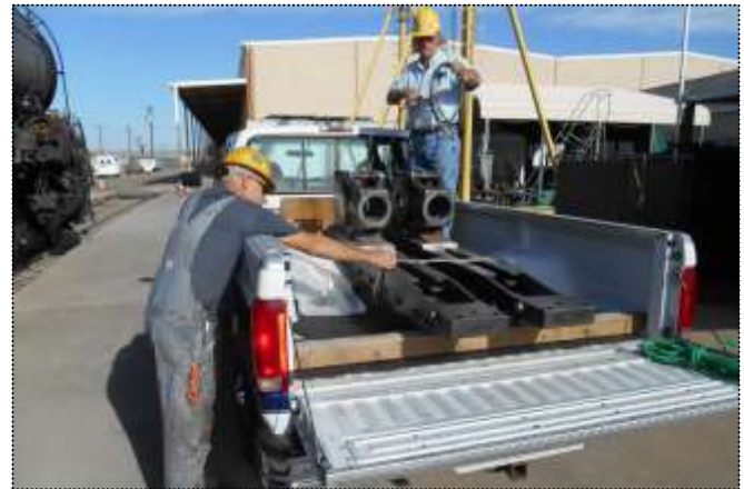
Left, GCRY Shop, Williams AZ: The refurbished crosshead assemblies are strapped into Rick Kirby's Ford truck. Right, Back Home: Unstrapping the load next to 2926 at the restoration site. The crossheads weigh 1450 pounds each.. Rich said that with a ton and one-half load, the Ford 250 Super Duty rode as smooth as a limo.
