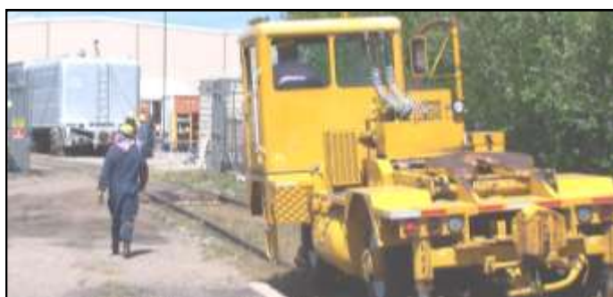
TILT, That's Not An Overweight Driver: Lurch the car mover leans left in this photo from May 2005 revealing the sad condition of the older portion of the spur. Though heavy, Lurch is a feather-weight compared to the locomotive and tender. The spur must be repaired before removing 2926 from the restoration site.
