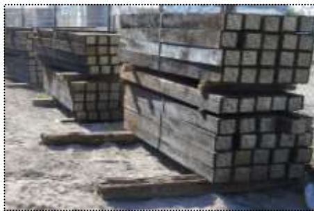
New ties with aroma of creosote.
