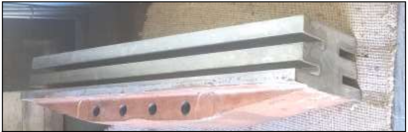
A restored shoe ready to reinstall: The precisely machined Babbitt grooves look like new, and should provide miles of smooth performance. Copper plating that was used as a base metal for the Babbitt is visible on the bottom of the shoe.
