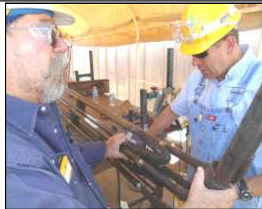
Left: Closeup of the firebox end of a superheater pair and the crew at work on the front end. Right: Carlos Osuna and Chuck Mangold. This is a different kind of superpower than recently retired Chuck was familiar with in C-130J aircraft.
