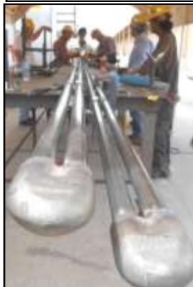
Left: Closeup of the firebox end of a superheater pair and the crew at work on the front end. Right: Carlos Osuna and Chuck Mangold. This is a different kind of superpower than recently retired Chuck was familiar with in C-130J aircraft.
